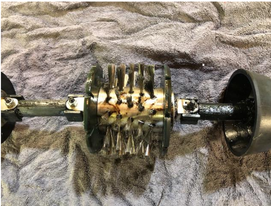
Figure 12--Brush Section of Cleaning Tool After Being Run in the Pipeline
