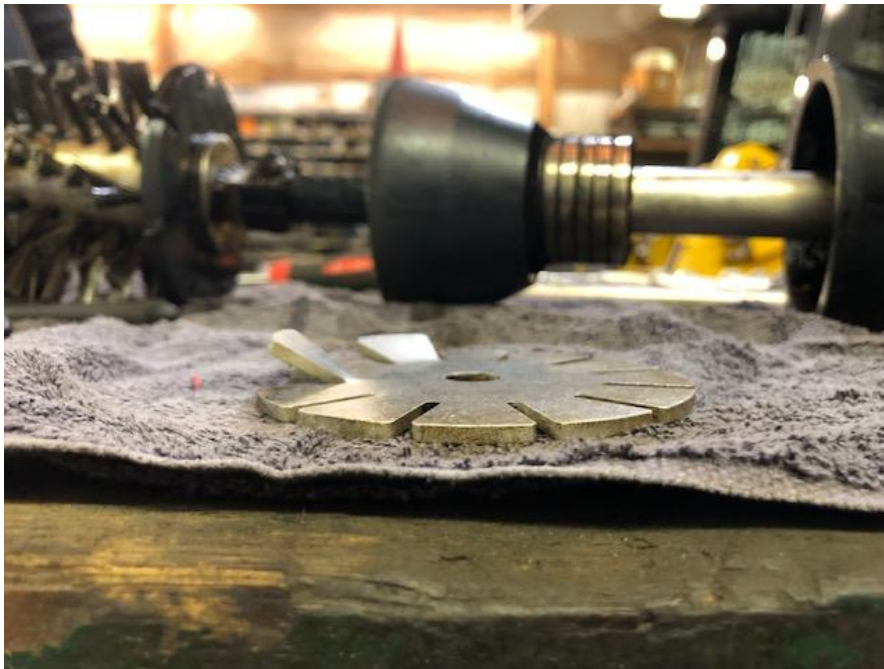
Figure 14--Gauge Plate with Bent Tabs
