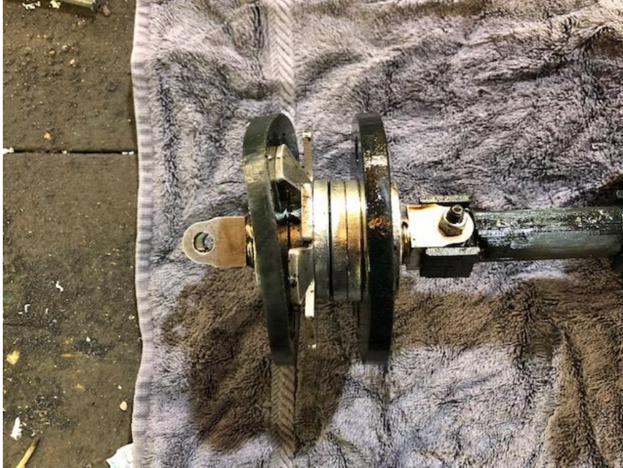
Figure 13--Gauge Plate Section of Cleaning Tool with Bent Tabs
