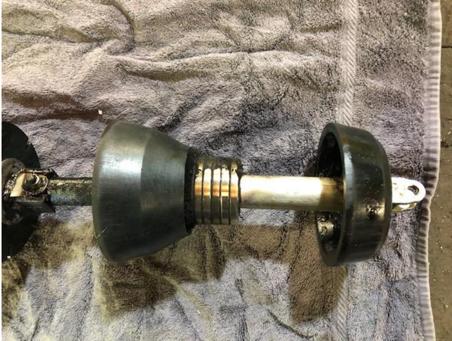
Figure 11--Drive Section of Cleaning Tool with Magnet After Being Run in the Pipeline
