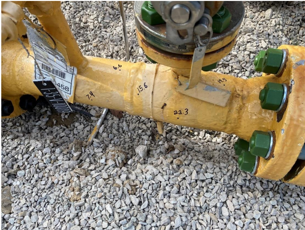
Figure 18--3" Heavy Wall Tee With Wall Thickness Up To 22.3mm(0.877")
