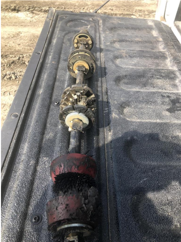
Figure 10 KMAX Cleaning/Gauge Pig with Magnets, Brush, Gauge Plate, and 22hz transmitter
