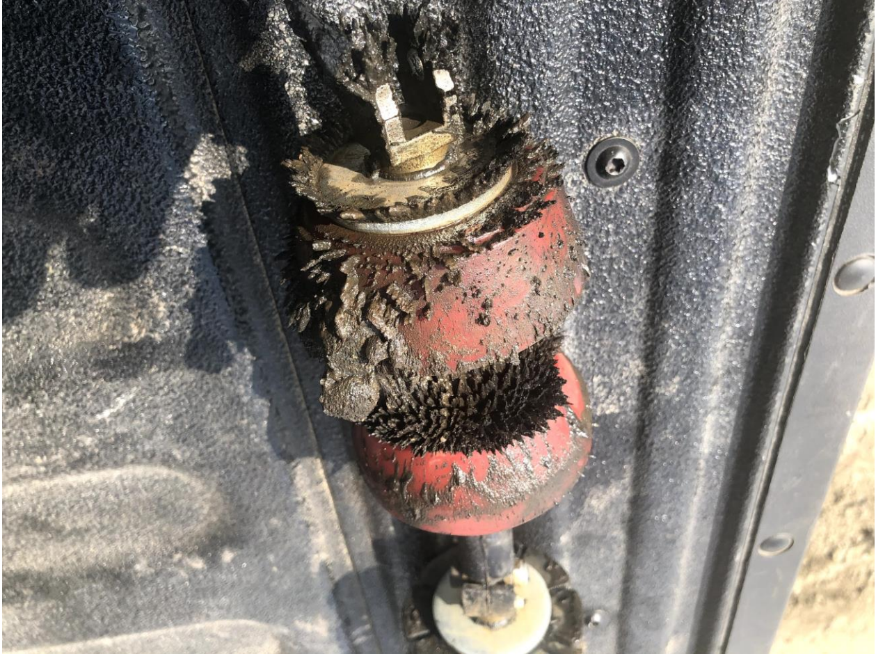
Figure 11 Debris on Magnets of Cleaning Pig
