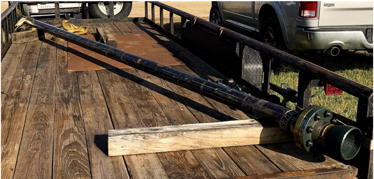
Figure 8 Calibration Spool of 4" Sch. 40 Pipe
